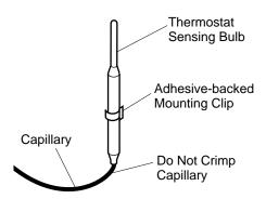
Figure 36 - Positioning the Thermostat Sensing Bulb in the Vertical Position with the Capillary at the Bottom
